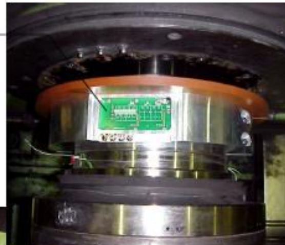
Telemetry Transmitter with T/C Connection Terminals
