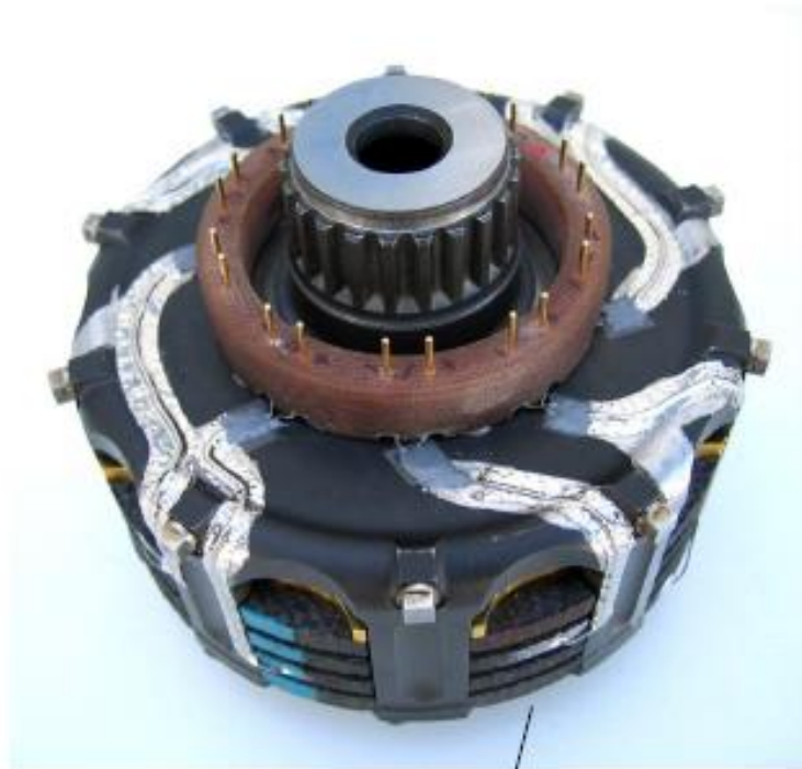
Instrumented Clutch Assembly with Sensor Connector Interface
