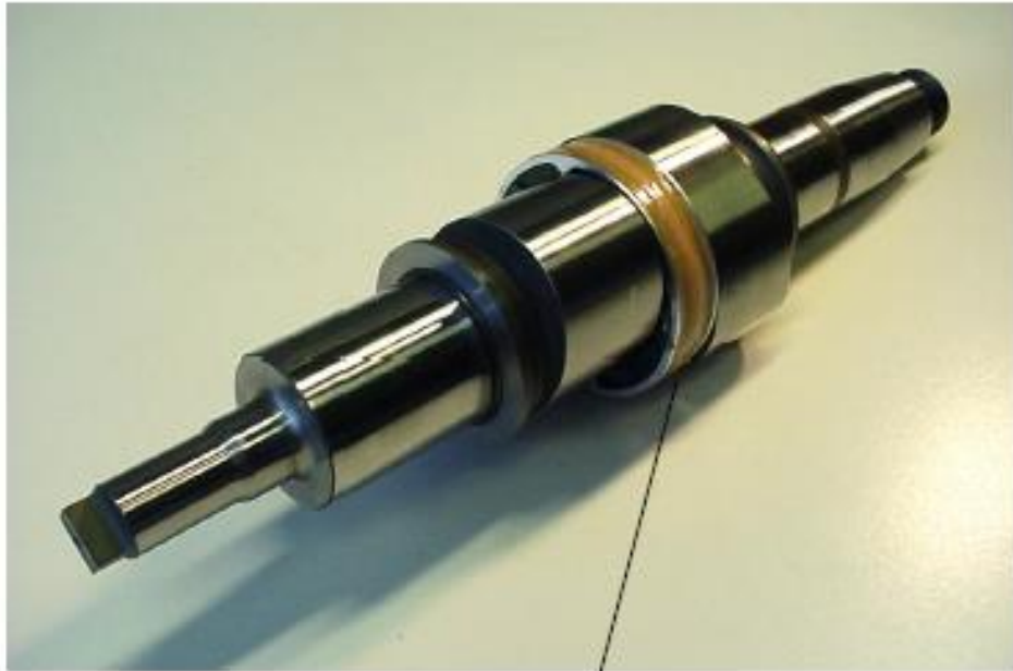
Custom Designed Telemetry Transmitter on Instrumented Shaft
