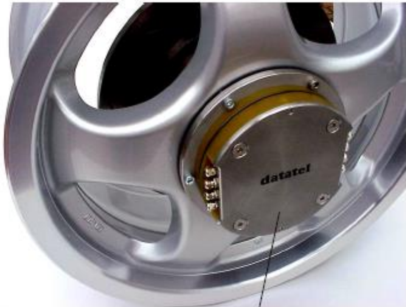
Transmitter Carrier installed on Wheel
